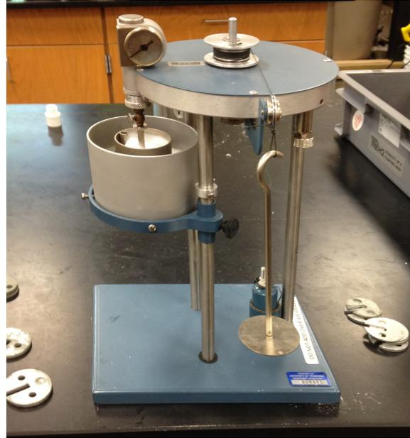
Figure 3. Thomas-Stormer Rotating Drum Viscometer
